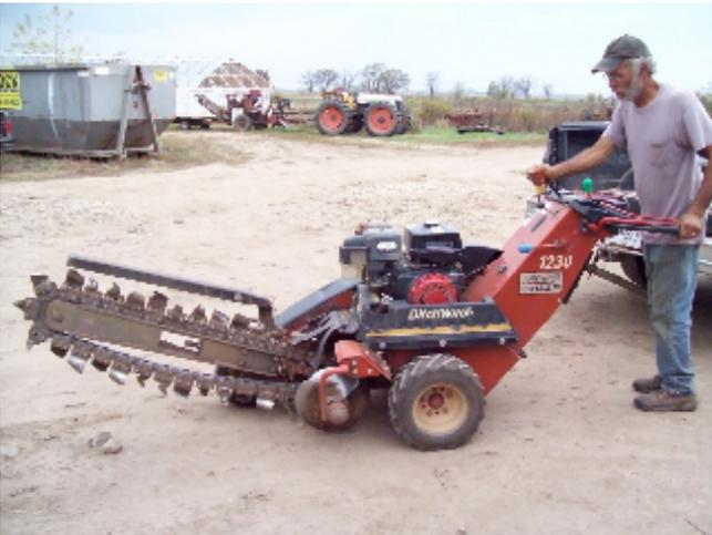
(left) We are in the midst of building a new greenhouse. Steve rented a trencher to bury the electric lines. While we had the trencher, he also laid water lines to each of our four greenhouses. We have a good water supply to the greenhouse area, but have used garden hoses to deliver water to each individual house. We will enjoy having a faucet in each greenhouse.
